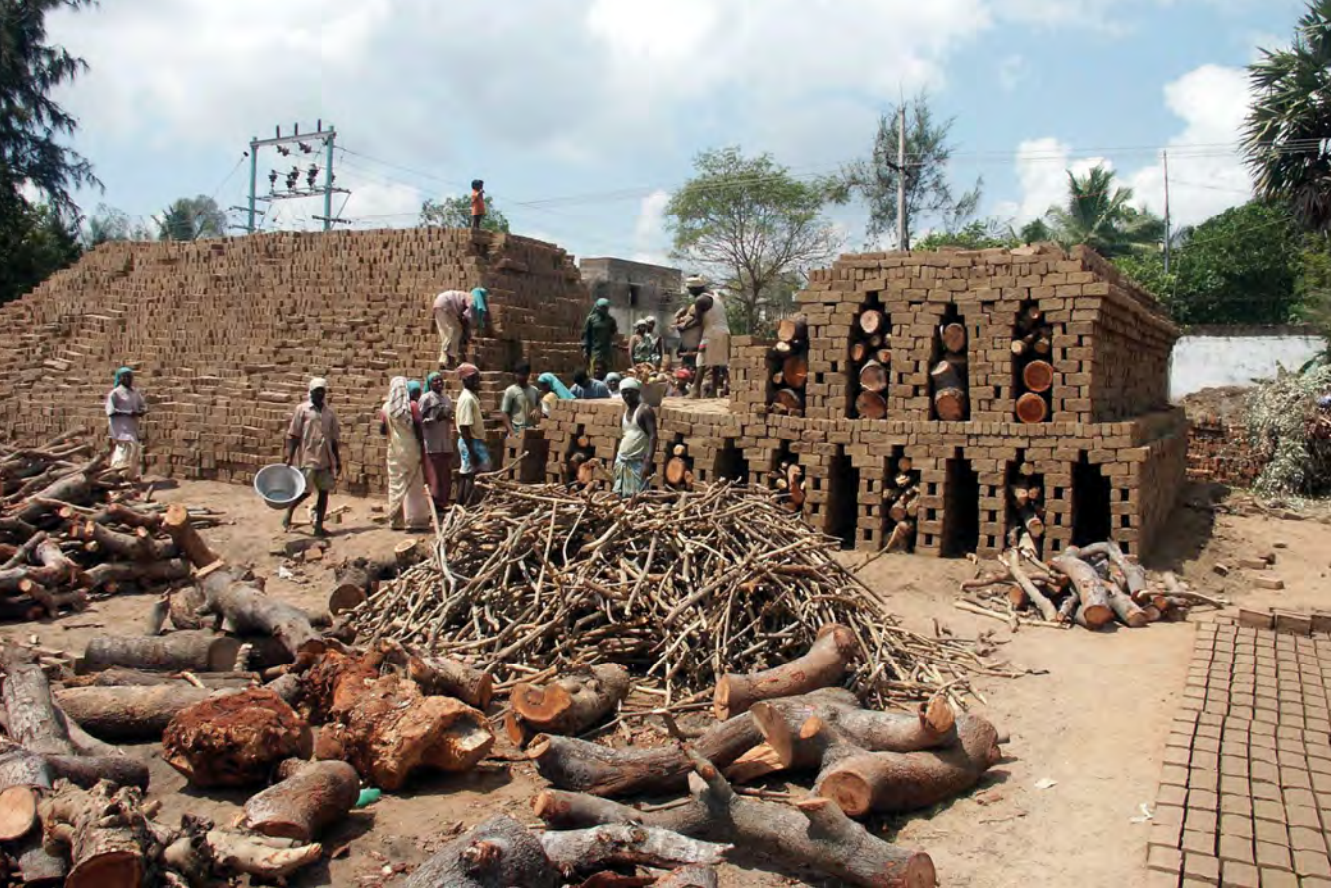
Figure 129—CFB industry in Pondicherry, Tamil Nadu: No management of material and fuel resources (Photo: Satprem Maini)
