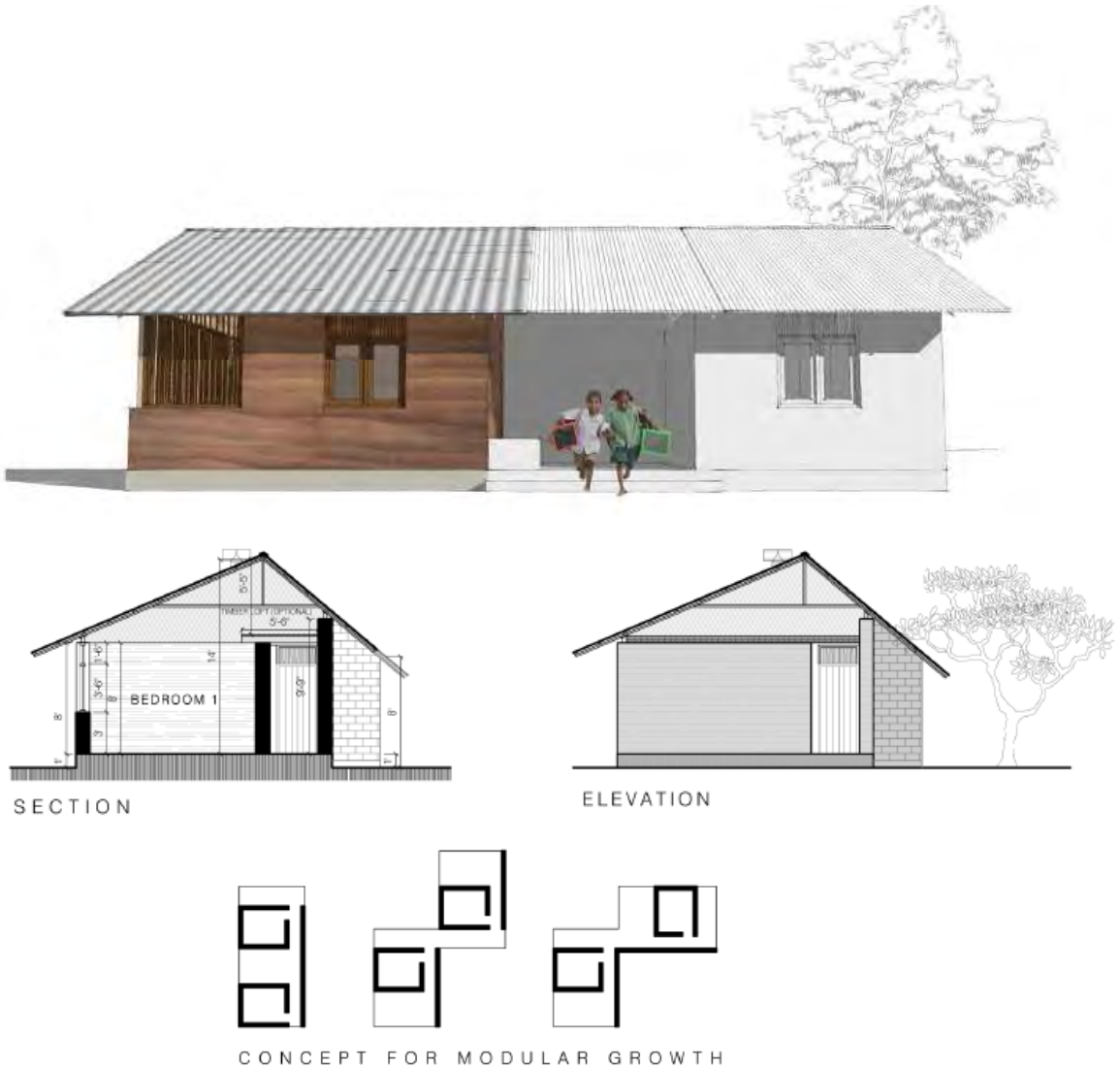
Figure 102—Tentative proposal of a rammed-earth house with a lockable core bedroom, a kitchen, chimney and toilet, which comprises a typical module that can be repeated in different alignments in incremental stages. (Source: HFHSL)
