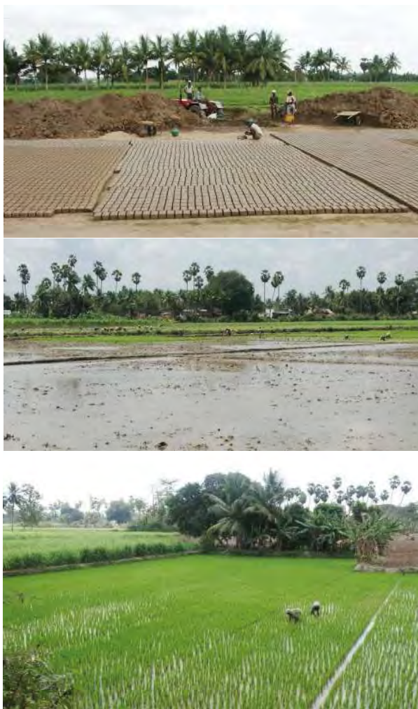
Figure 140—Sustainable CFB production. Excavation for the production of bricks, Flooding of fields and excavation converted into agricultural rice fields. (Photo: Satprem Maini)
