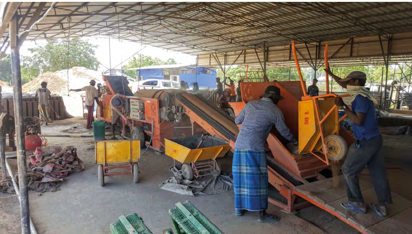
Figure 105—Hydraulic CSEB machine in production yard in Batticaloa district, managed by HfH and WV and funded by the EU. (Source: Jaime Royo-Olid, EU 2018)
