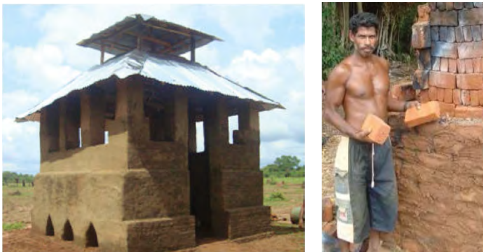
Figure 189—An improved brick kiln in Vavuniya and a trained burnt brick producer in Vavuniya showing his products (Source: Practical Action)
