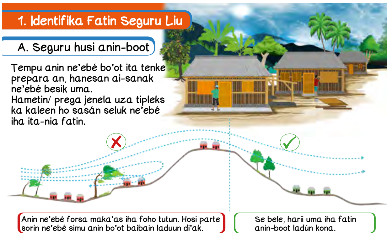
Fig. 13: National Shelter Manual," page 5. Guidance on securing houses against strong winds by maintaining a safe distance from trees and reinforcing structures using appropriate materials for protection during disasters.
