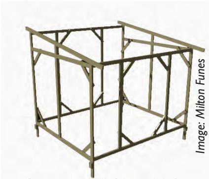
Computer model of the timber frame of the shelter
