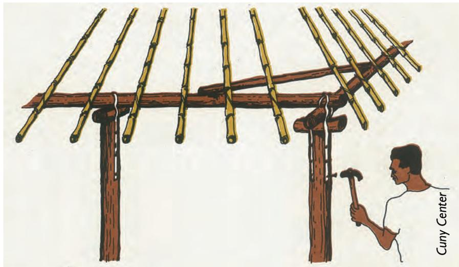
Safer shelter techniques - strapping columns to beams
