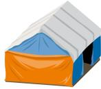
**EMERGENCY SHELTER** consists primarily of tarpaulins and fixings such as ropes, nails, a hammer etc. Tents can also be used for emergency shelter but, because they are less versatile than tarps, their use is limited. Emergency shelter can be distributed quickly but offers only limited protection against heavy rains.
