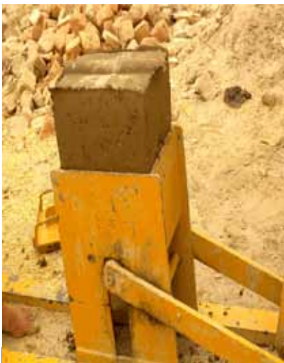
Compressed mud blocks were abandoned after the pilot stage due to a lack of community acceptance and slow production speed. Photo: ACTED
