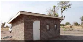
Approximately 25 per cent of the shelters were built using compressed soil blocks. The technique represented a financial and environmental improvement, but was slower, requiring significant efforts to introduce as a new technology. Photo: Fernando Murillo
