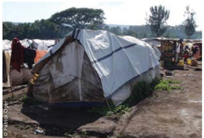
A good-quality tarpaulin can resist up to a year or longer. It can be used for multiple purposes, such as covering older plastic sheets to provide waterproofing.
