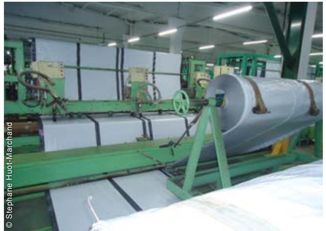
Suppliers started producing the new tarpaulin in the late 1990s. The use of reinforcement bands instead of eyelets allows for mechanization, increasing quality and speed of production.
