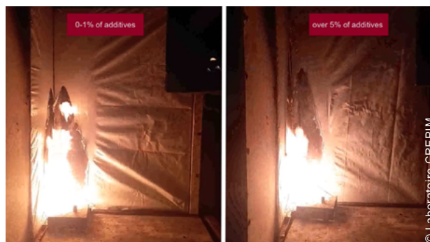
Fire resistance testing showed the feasibility of the new specification, even without the use of fire-retardant additives.
