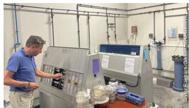
UV testing was essential for the new specification development, as durability largely depends on the capacity of the tarps to withstand solar radiation.
