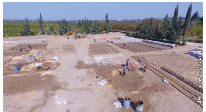
Adobe brick production required very large spaces and could only be conducted during the dry season. This caused some implementation challenges.
