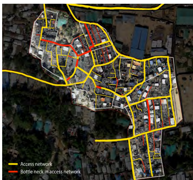
A map of the 'Existing Access Network' with network bottlenecks prepared in order to address them by replanning. (Second fire response, January 2022).
